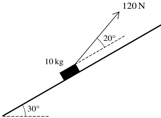
A block of mass 10 kg is at rest on a rough plane inclined at an angle of  $30^\circ$  to the horizontal. A force of 120 N is applied to the block at an angle of  $20^\circ$  above a line of greatest slope (see diagram). There is a force resisting the motion of the block and 200 J of work is done against this force when the block has moved a distance of 5 m up the plane from rest.
