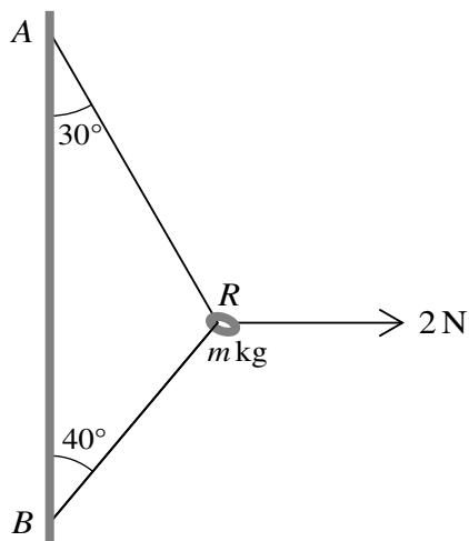
The diagram shows a smooth ring  $R$ , of mass  $m$  kg, threaded on a light inextensible string. A horizontal force of magnitude 2 N acts on  $R$ . The ends of the string are attached to fixed points  $A$  and  $B$  on a vertical wall. The part  $AR$  of the string makes an angle of  $30^\circ$  with the vertical, the part  $BR$  makes an angle of  $40^\circ$  with the vertical and the string is taut. The ring is in equilibrium.
